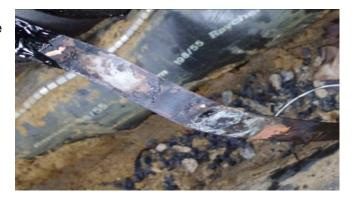
Reinforcing tape failure results in the lead sheath being unable to contain the oil pressure, leading to 'bulging' of the sheath and, eventually, oil leaking from the cable causing environmental and reliability performance issues.
