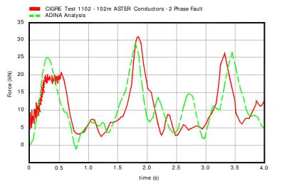
Correlation between full-scale test data (CIGRE technique) and Dynamic Analysis Technique results (ADINA new technique)
