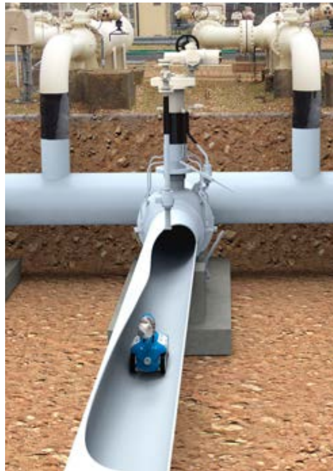
A magnetised track system will keep the GRAID robot firmly fastened to the pipe wall, but also give it the flexibility to drive freely
